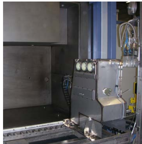
Figure 3: SF 6 filling Station and Tightness test tank
