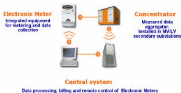
Fig.4 The Automatic Meter Management system
