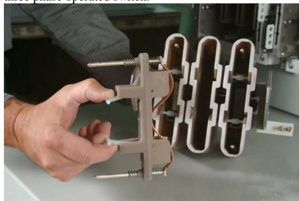
Fig. 3: Contact bridge of Magnefix MA
