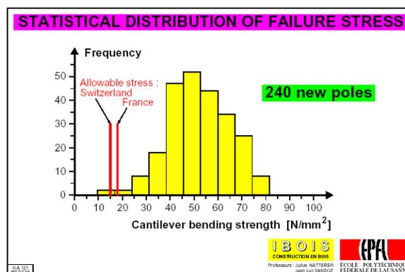
**Figure 1:** 240 new wooden poles tested until failure to determine the Cantilever bending strength (Spruce and Fir). IBOIS database, Swiss Federal Institute of Technology, Lausanne
