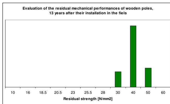
**Figure 9:** Non-destructive evaluation of residual mechanical bending strengths of wooden poles, 13 years
