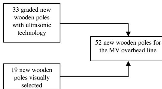
**Figure 7:** Selection of 52 new wooden poles for a MV overhead line construction: 33 poles are graded thanks to the ultrasonic non-destructive method, 19 poles are visually selected.
