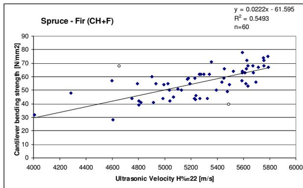
**Figure 3:** Non-destructive evaluation of new wood poles mechanical properties. Sylvastest Trio technology. Ultrasonic velocity vs. Cantilever bending strength. Spruce-Fir. Left: destructive tests in laboratory.
