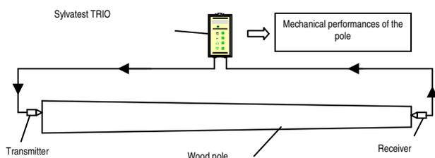
**Figure 2:** Concept of the ultrasonic measurement for a new wooden pole. One emitter and one receiver: measurement of the time of flight of ultrasonic waves.
