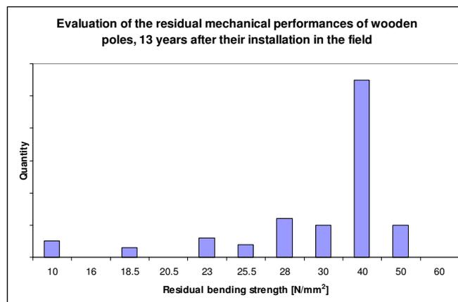
**Figure 8:** Non-destructive evaluation of residual mechanical bending strengths of wooden poles, 13 years after their installation in the field. Spruce-Fir, CCB Switzerland. All the poles.
