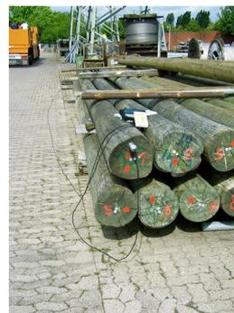
**Figure 4:** New-wooden-poles quality evaluation using Sylvastest Duo. Inspection in Germany (Fir-Spruce).
