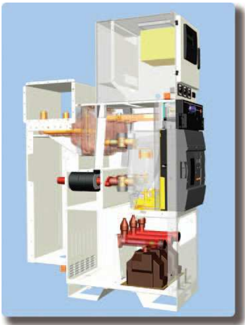
Figure 3: size of the metering unit can be reduced to 375 X 900 X900 mm
