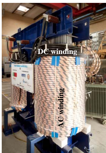
Figure 7 A fault-current limiter (FCL) with common core and trifilar windings undergoing asymmetric behaviour characterisation in the FPGLab
