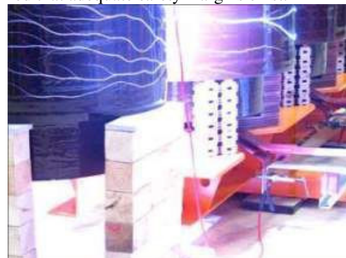
Fig. 7: 72.5 kV dry-type transformer prototype being tested to the limit.
