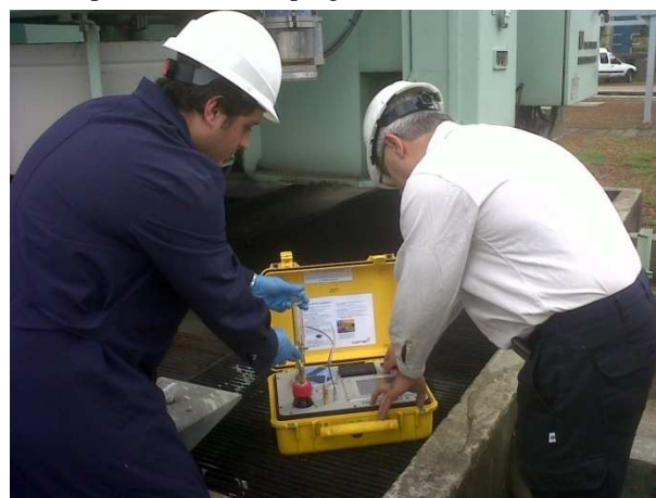
Fig. 2 - Gas-in-oil content analysis in field.
