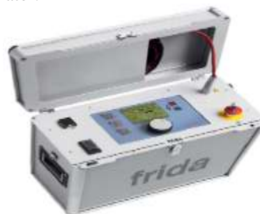
Fig. 1: Portable VLF test set This generator has a very low noise level, so sensitive PD
