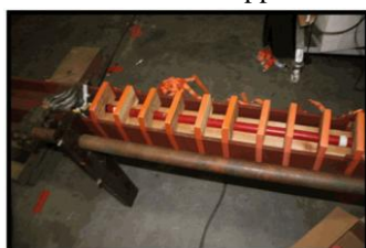
Figure 5: Cables maintained by wooden pieces
