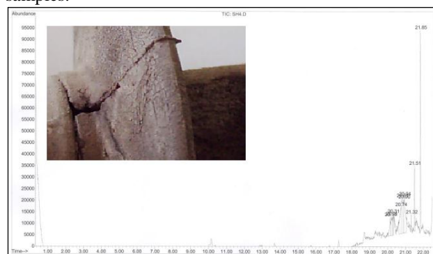
Fig8: gas chromatograms for composite insulator sample
