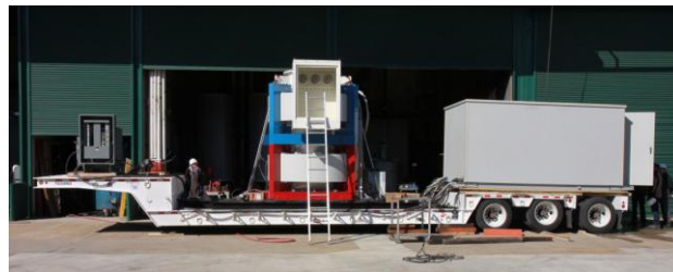
Figure 5 SFCL at KEMA Powertest
