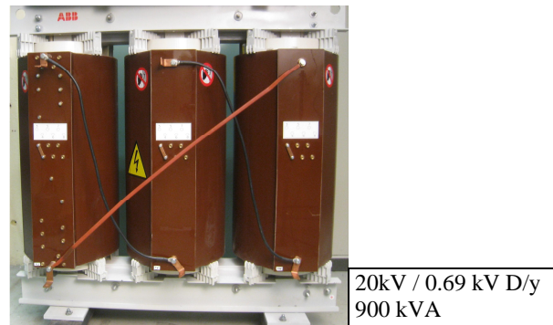
Figure 1. Test transformer with measuring taps along one of the high-voltage windings.
