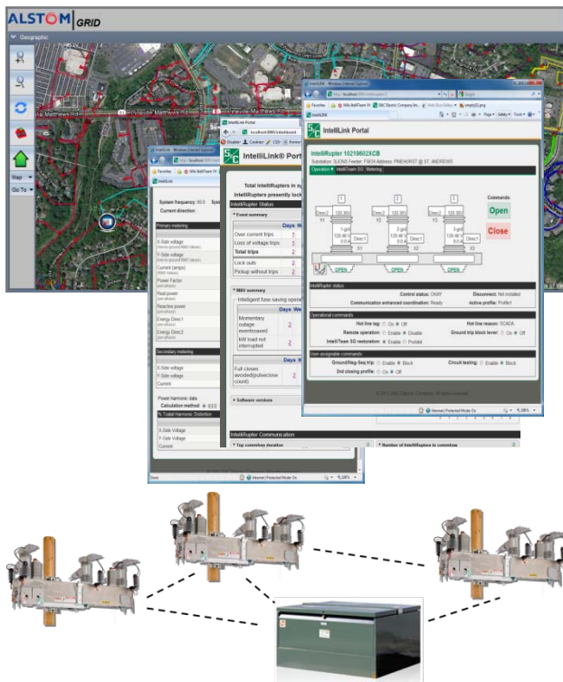
Figure 1. Layered Intelligence - Central Intelligence (IDMS), regional intelligence (performance dashboards and device drilldown), and local /distributed intelligence (protection and switching devices).
