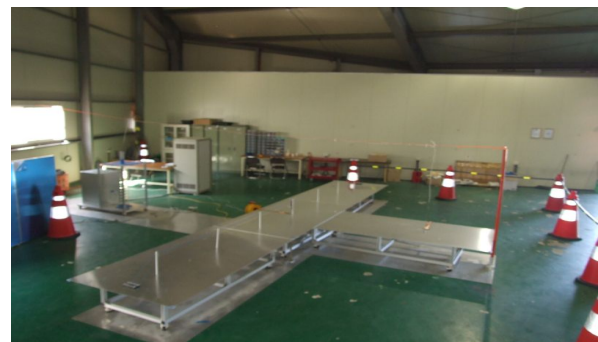
Fig. 4 Simulation line for the down scaled simulation test (50:1)
