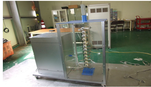
Fig. 3 Impulse generator used for the down scaled simulation test
