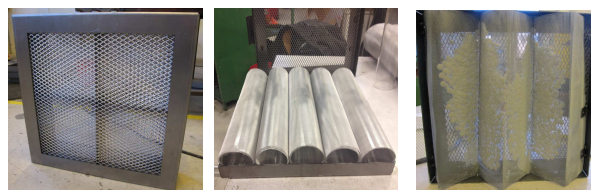
Figure 3. Left: Front view of absorber with expanded metal of aluminium for test 2. Middle: Open absorber showing an arrangement of rolls (with 10 layers) of expanded metal in test 4. Right: Open absorber showing an arrangement of expanded steel mesh with boric acid tablets in test 6.
