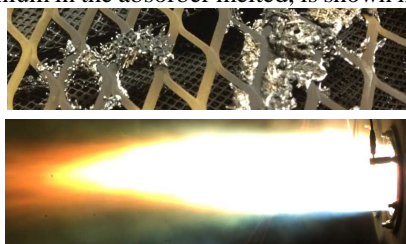
Figure 5 Above: Melted aluminum on expanded mesh of steel from test 4. Below: Hot gas jet with length of 450 mm escaping through relief openings from arc compartment in test 1 without buffer, high speed camera exposure.
