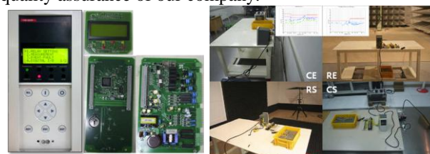
Fig. 7: The appearance of the high speed OCR and photograph of the EMI/EMC tests
