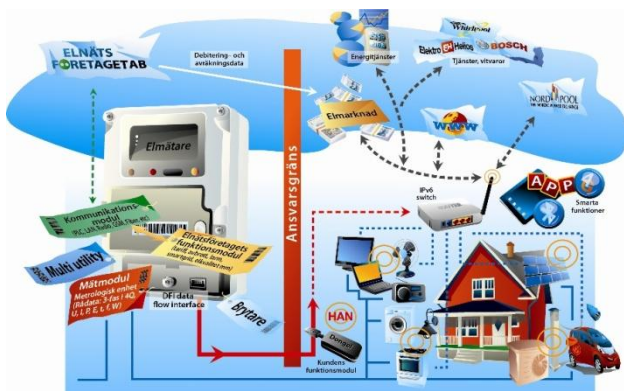
Figure: The DFI interface provides consumption data in real time. Price information is imported from the internet to a residential gateway owned by the electricity consumer.
