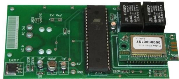
Figure 4: The hardware design for a socket node
