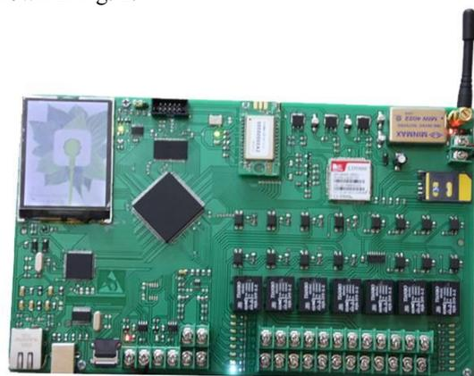
Figure 2: The hardware design of a coordinator node
