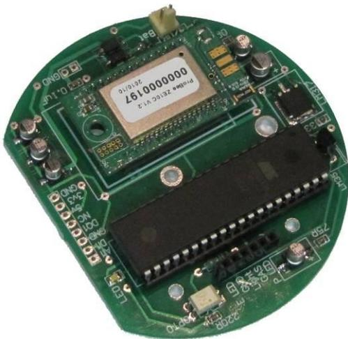
Figure 3: The hardware design of a sensor node
