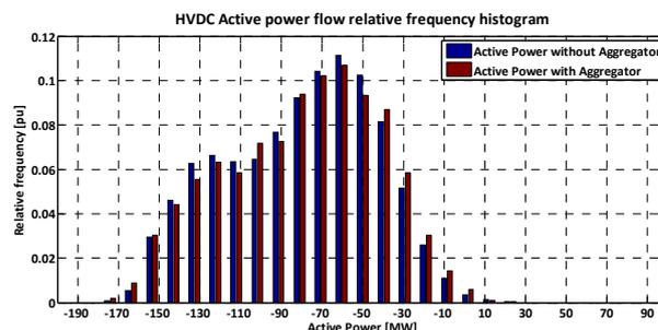
Fig. 1. Relative frequency histogram of the power flow on the HVDC cable during the heating season with and without the aggregator assuming the adoption of the wind following strategy in the 100% wind penetration scenario.
