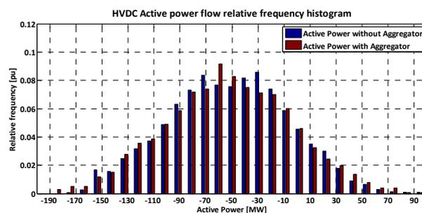
Fig. 4. Relative frequency histogram of the power flow on the HVDC cable during the heating season with and without the aggregator assuming the adoption of the price following strategy in the 100% wind penetration scenario.
