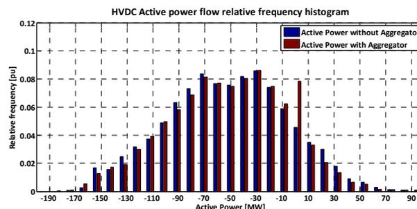
Fig. 3. Relative frequency histogram of the power flow on the HVDC cable during the heating season with and without the aggregator assuming the adoption of the wind following strategy in the 200% wind penetration scenario.
