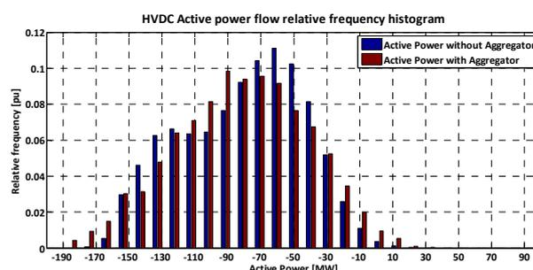
Fig. 2. Relative frequency histogram of the power flow on the HVDC cable during the heating season with and without the aggregator assuming the adoption of the price following strategy in the 100% wind penetration scenario.
