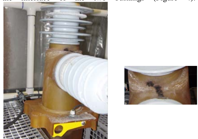
Figure 4: Salt Spray Test of Prototype Housing made out of urethane
