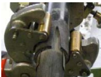
Fig. 5: Closing oversheath on the copper plate with a roll-tool
