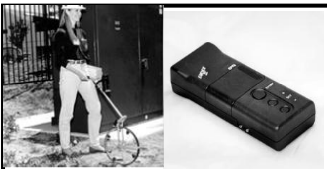
Figure 1: EMDEX II Meter and Linear Data Acquisition (LINDA) Wheel
