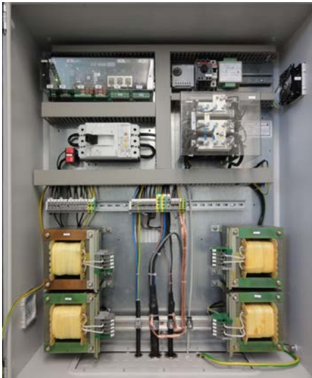
Fig. 7. Realized thyristor controlled High-Power-Current-Injection (HPCI)
