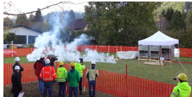
Fig. 8. Field test with 10m OHL-conductor lying on ground, 20kV-network, I_{ce} = 115 A, 30 A overcompensation
