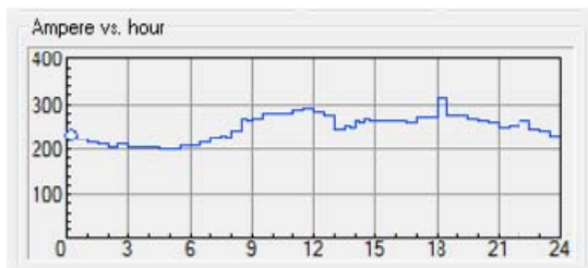
Figure 1 – Example of a load diagram calculated by the chronological power-flow in DPlan
