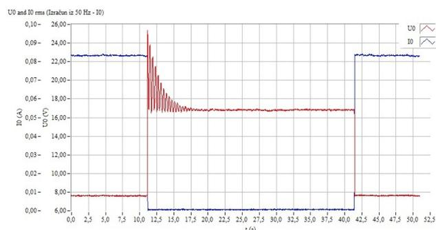
Figure 3: Recording of current and voltage measurement at breaking of NGR
