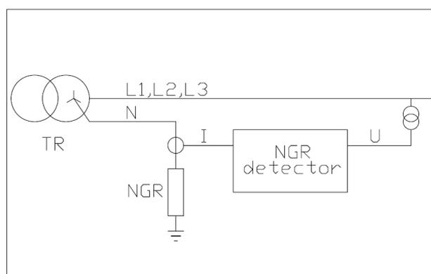
Figure 1: Connection diagram ( $I$  - current through NGR,  $U$  - residual voltage)
