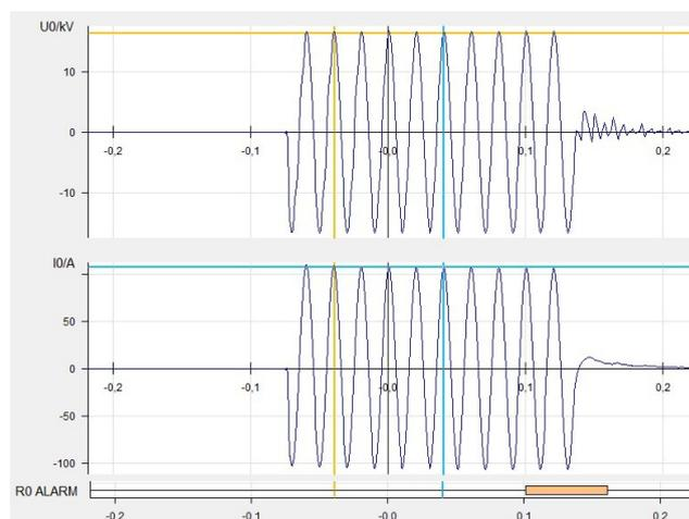
Figure 4: Recording of current and voltage measurement and alarm trigger at ground fault by higher resistance of 160  $\Omega$
