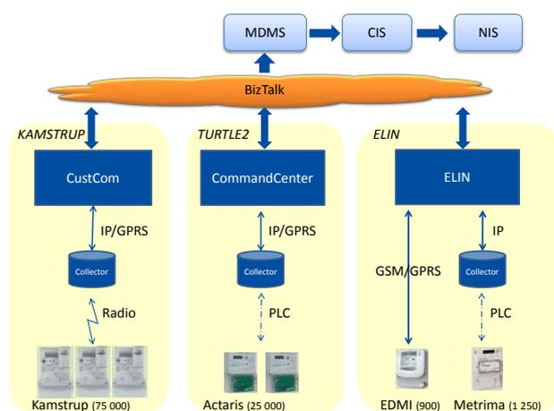
Figure 1. AMI solution at Mälarenergi (in-house)
