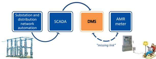
**Figure 2.** AMR is the missing link in order to control LV network from DMS system
