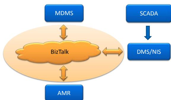
**Figure 3.** System overview of integration between AMR meters and DMS/NIS
