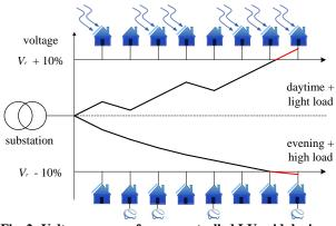
Fig. 2: Voltage curves of an uncontrolled LV grid during a sunny day and in the evening
