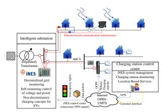
Fig. 4: Concept of the intelligent integration of electric vehicles
