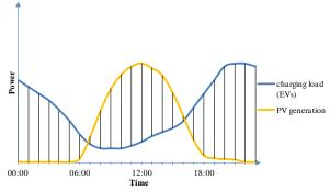
Fig. 1: Comparison of a characteristic PV generation and a cumulative EV charging load
