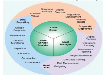
Figure 1. Asset management is based on three functions (asset owner, asset manager, and asset service provider), a single process, and many decisions.[1]
