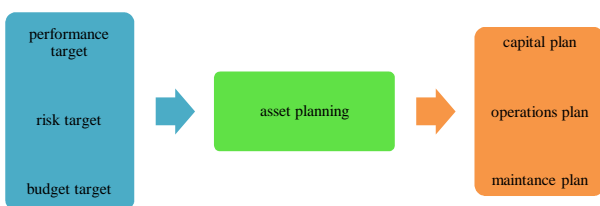
Figure 5: Asset planning identifies the best combination of capital, operations, and maintenance spending to achieve all targets for the least possible life-cycle cost.
