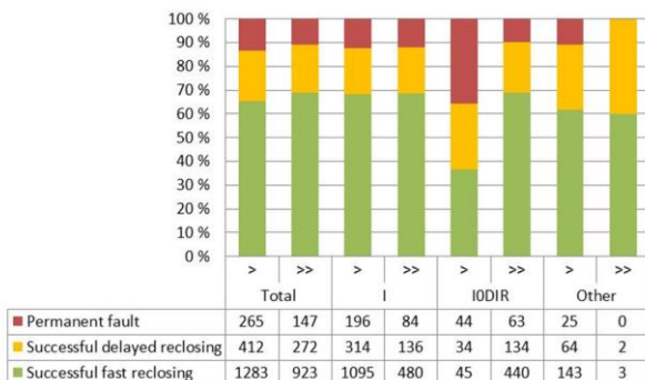
Figure 7. Success rate of reclosings according tripping threshold level and reason of tripping
