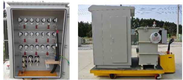
Figure 11. Variable load and fault generator
