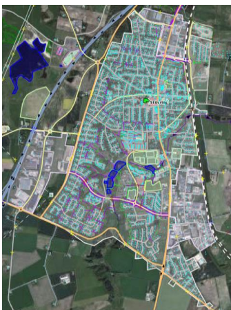
Figure 3: City in Simulator with DER shown as Dots Furthermore a real-time digital simulator is utilized to recreate a benchmark grid, in this case the electrical grid of the town of Støvring in Denmark. It serves as an area
