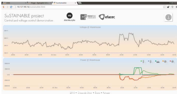
Figure 6 – Detailed voltage and load profiles
