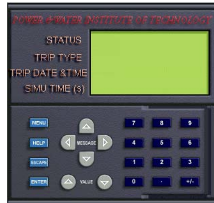
Figure 1: Developed multifunctional microprocessor based subsystem in MATLAB/Simulink environment.
