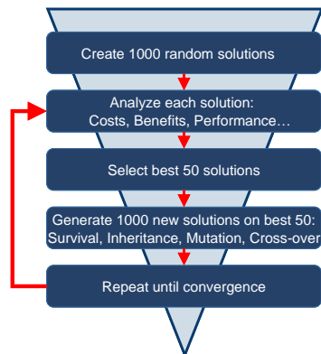
Figure 4: Principle of genetic algorithm
