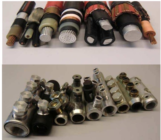
Fig. 12: from paper 290, a few representatives of MV cables and mechanical connectors
