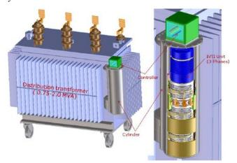
Fig 25: from paper 0580 – Example IVTI mounted on distribution transformer
