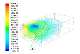
**Fig. 30:** from paper 1301 - CFD simulation showing a pressure peak in the corner of the switchgear room 17 ms after the fault initiation
