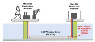
Fig. 2: from paper 1334 – Subsea circuit overview
