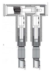
**Fig. 10:** from paper 1288 – Cross-section of two stacked, unscreened connectors with integrated earthing bolt
