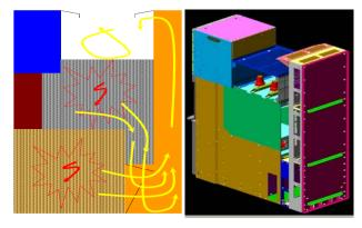
**Fig. 31:** from paper 1057 – Example of introverted release in case of internal arc fault
