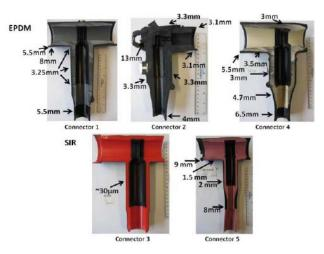
**Fig. 7:** from paper 1341 – Section of the connectors illustrating their design
