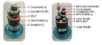
**Fig. 24:** from paper 0951 – Composite cables design and configuration of cable joint
