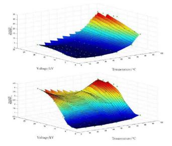
**Fig. 4:** from paper  $1258 - Tan(\delta)$  fingerprints of a sample that has been in operation for over 40 years (top) and of a sample that has been in operation for over 20 years (bottom)
