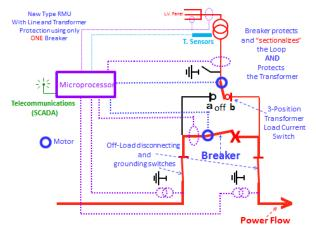
**Fig. 33:** from paper 0274 – Single line diagram of "smarter RMU"
