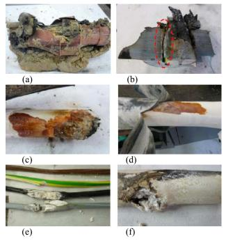
**Fig. 6:** from paper 0581 – (a) resin not correctly poured; (b) poor adhesion between the resin and the XLPE insulation; (c) & (d) corrosion on the PVC filler; (e) corrosion of conductors; (f) degradation due to water ingress
