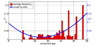
**Fig. 16:** from paper 1321 – Age-related damage frequency per year and model function (bathtub curve) of low-oil-content circuit-breakers
