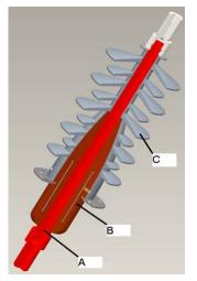
Fig. 36: from paper 1219 – Combined insulation bushing
