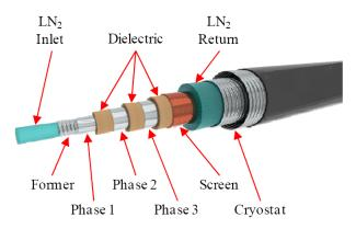
**Fig. 26:** from paper 0742 – HTS cable design for the AmpaCity project
