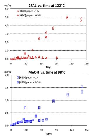
**Fig. 8:** from paper 0407 – Evolution of the 2-FAL at 122°C and MeOH at 98°C (in ppm) with different initial levels of water content in the paper
