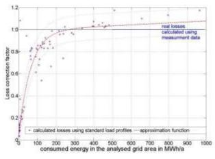
Fig. 1.7: Loss calculation correction factor (paper 1186).
