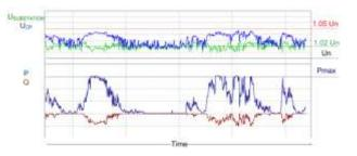
Fig. 2.8: DG voltage control (regulating Q) with droop and deadband (paper 0494).
