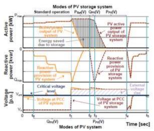
Fig. 2.9: comparison of voltage control strategies for PV and PV storage systems (paper 1396).
