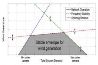
Fig. 1.16: Stable envelope for wind generation operation on Shetland (UK) power system (paper 1381).
