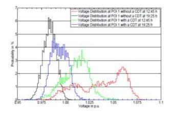
Fig. 1.4: Impact of Controllable Distribution Transformer on voltage probability in LV network (paper 0575).
