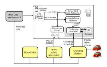
Fig. 2.5: Low Voltage Grid Controller architecture (paper 1268).
