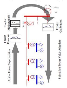
Fig. 2.4: RiesLing - Power flow forecast and calibration process (paper 0316).
