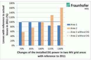
Fig. 1.8: MV system losses variation with DG penetration (paper 1478).
