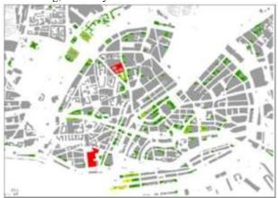
Fig. 3-8: Map section of Hamburg displaying the demand side integration potential for HVAC in office-like buildings (paper 1436).
