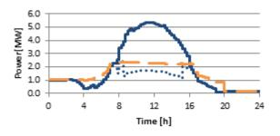
Fig. 2.2: DG grid infeed before curtailment (solid line) and optimised VPP management of DG (dashed line) in comparison to standard curtailment measures (dotted line) (paper 0785).
